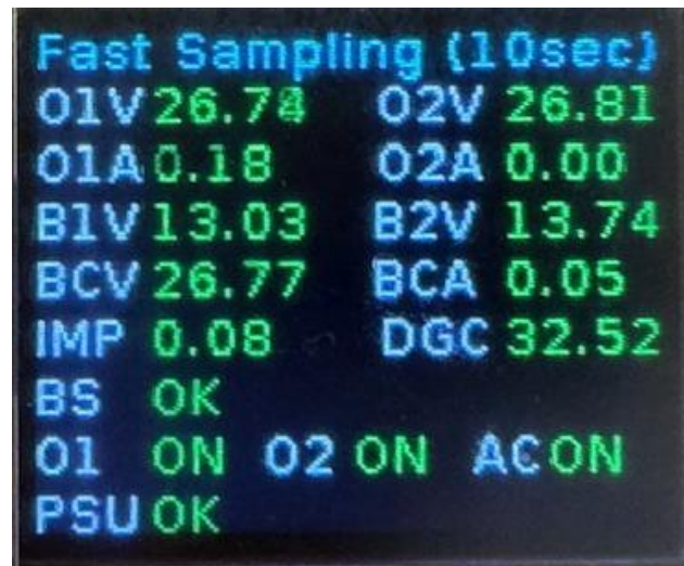
High speed sampling rate displays peak-to-peak voltages and current outputs of the connected equipment.
